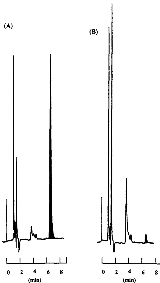
Figure 1 Representative chromatograms of DSG ( 0.5 \text{ mg ml}^{-1} ) in 0.05 \text{ M Na}_2\text{HPO}_4 , pH 11.5, at (A) the start of the stability experiment and (B) 4 min later.
